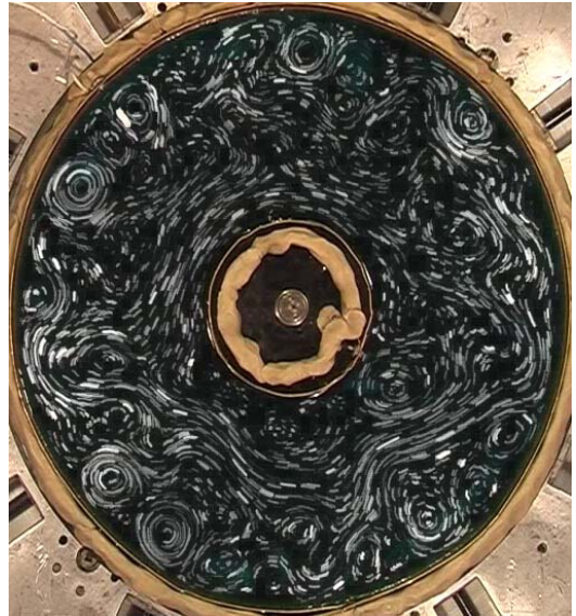
Well defined narrow jet flows, channel 2: a) h=24 mm, T=67.0 sec, b) T=39.8 sec, h=24 mm.
