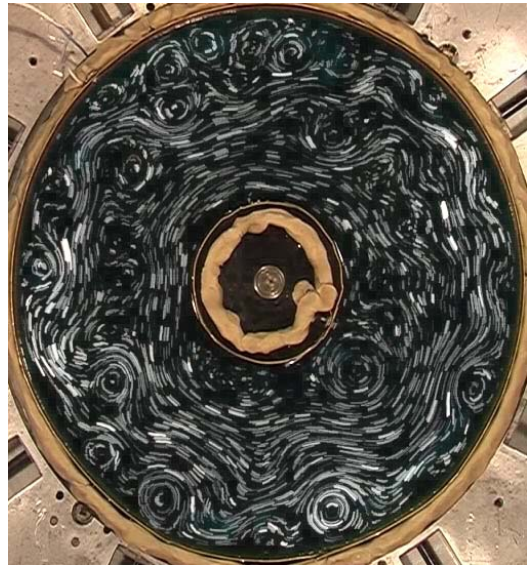
The jet flow in channel 2 (T=39.8 sec, h=24 mm) at different instants of time.
