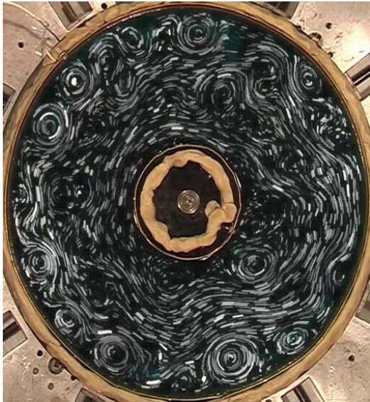
The jet flow in channel 2 (T=39.8 sec, h=24 mm) at different instants of time.
