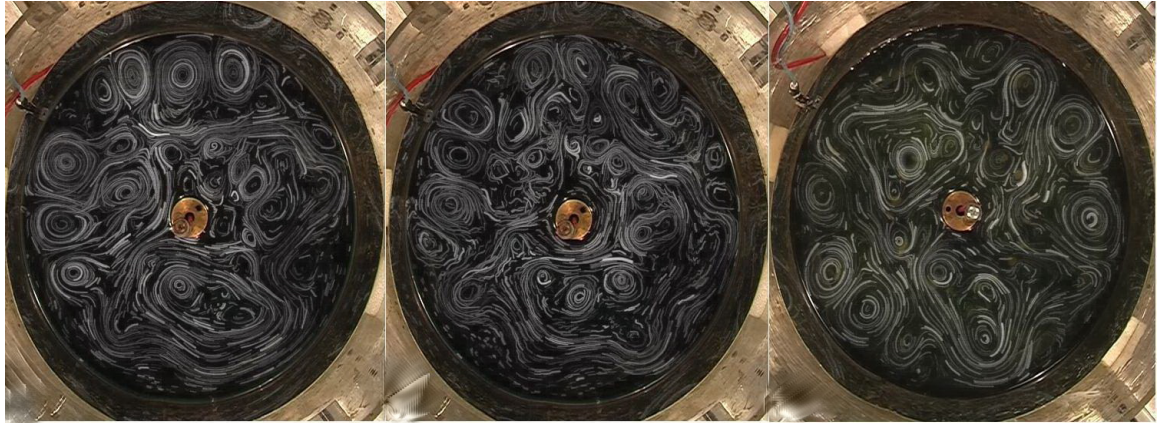
Particle trajectories during generation of vortices with formation of clusters by shear flow in channel 1: (a) T=15.4 sec; (b) another current direction T=15.4 sec; (c) T=19.1 sec.
